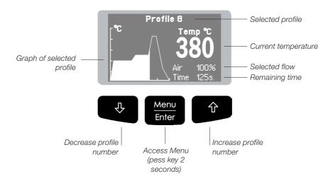
You can switch between operating modes (Manual Mode / Profile Mode) by pressing the "increase" and "decrease" keys simultaneously for 2 seconds. (Only if mode profiles is ON)
