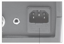
Remove the fuse by pulling the black cap. If necessary use a tool to lever it off.
